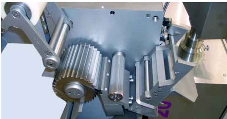
View into the cutting chamber
